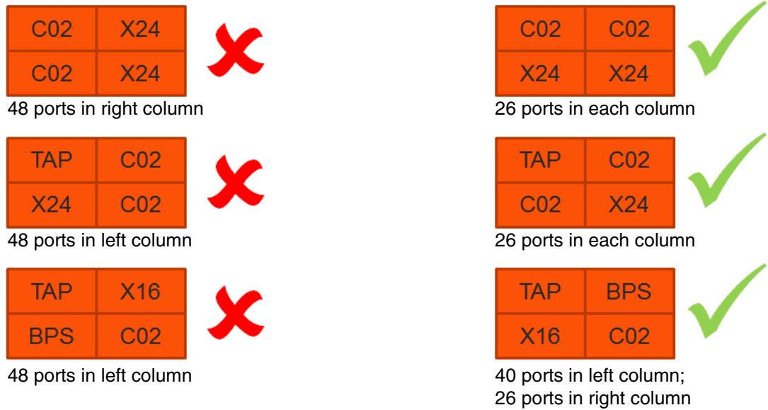
Figure 1-7: Module Placement of PRT-HC0-CO2, 100G Mode
